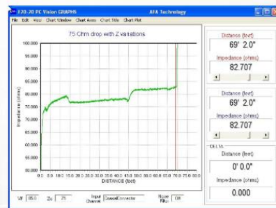
75 Ohm drop with impedance variations
