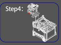
Place the fiber cleaver on the operating table, adjust the depth of the screw to make the rubber pad and the cleaver completely fit
