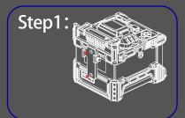
Fasten the fixing base to the back of the splicer with screws
