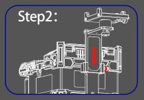
Insert the support frame into the socket of the base, adjust it to a proper height, and tighten the screws
