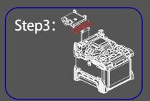
Place the cooling tray on the support frame, and make its hole position coincide with the point position on the support plate
