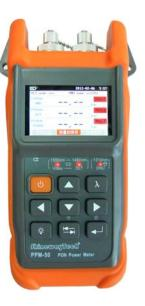
PPM-50 PON Power Meter can perform in-service testing of all PON signals (1310/1490/1550nm) on any spot of the network featuring pass-through design, burst mode and Pass/Warning/Fail assessment function, which can greatly help you evaluate PON signals transmission quality.
